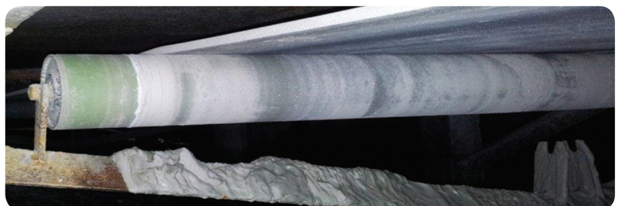
Single length Nylon or HDPE tube. (No weld joints)
