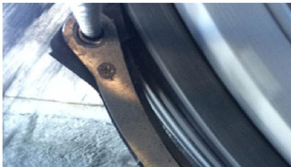
CleanScrape™ primary can be used on a wide range of applications i.e. Rubber or PVC, low or high speed, smooth or coarsely worn belts, caring dry, wet, fine, coarse, adverse chemicals and abrasive materials.
