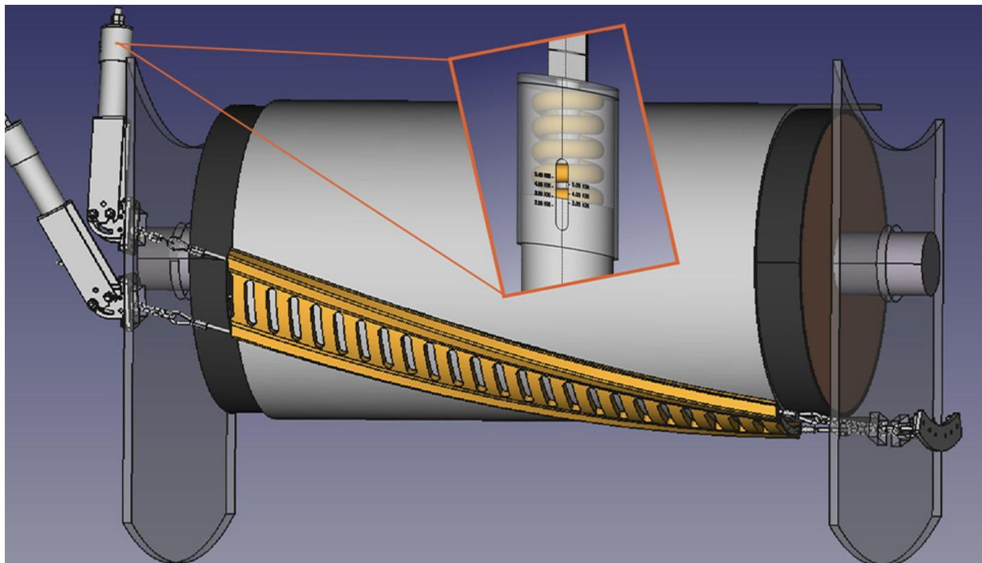
With its distinctive 3D helix design it is diagonally fitted to the discharge drum, and therefore always in touch with the conveyor belt independently of the belt contours.
